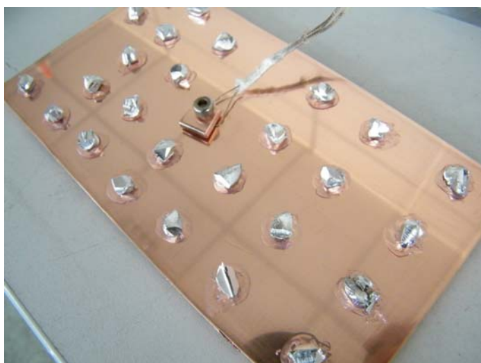
Fig.3.1 Assembly used for spread test
