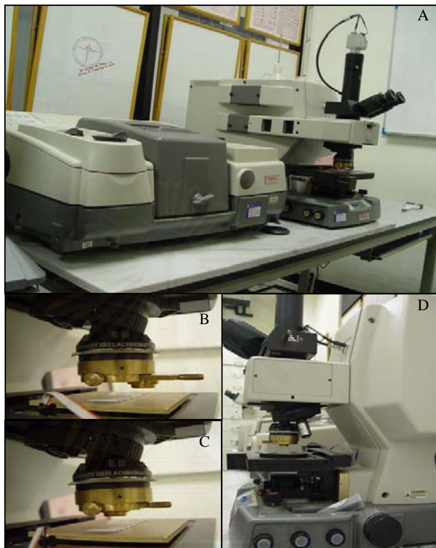
Figure 3.2 The homemade slide-on diamond \mu IRE was fixed on the 15X Schwarzschild-Cassegrain infrared objectives: (A) picture of Nicolet 6700 FT-IR spectrometer equipped with infrared microscope, (B) slide-on diamond \mu IRE was fixed on Continuum TM infrared microscope, (C) slide-on diamond \mu IRE was fixed on infrared microscope and aligned to high energy throughput, and (D) infrared microscope.
