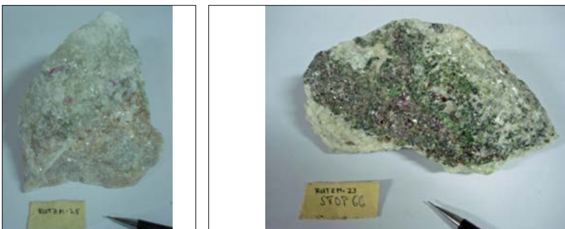
Fig. 4.2: The two samples from Visakazi II Mine represent two different zones in terms of production site as well as in terms of mineralisation. Sample WB1 is taken in the open pit operation of Visakazi II Mine and represents the neck of a mineralised boudin-shaped lense where as sample WB6 contains a core of such a lense which was collected in the drift operation at Visakazi II Mine.
