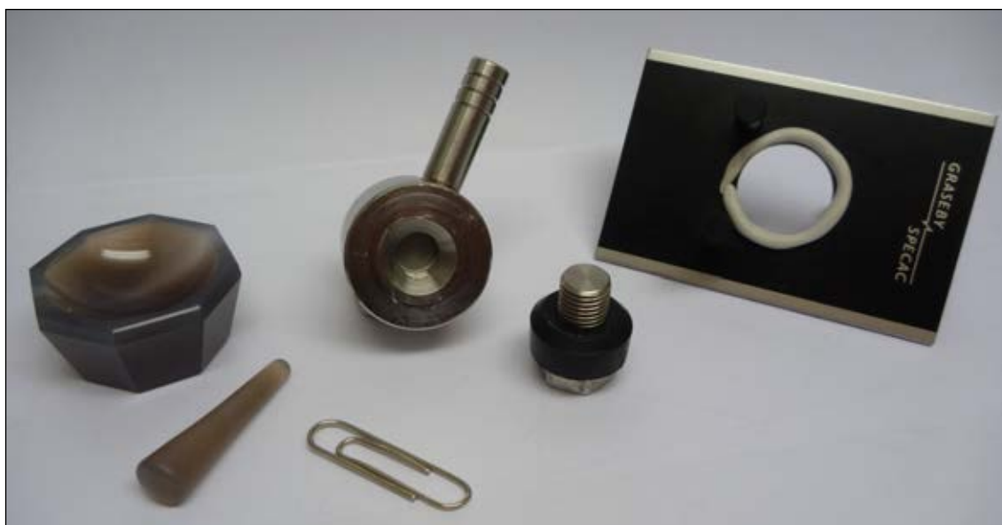
Fig. 1.2: Tools used to create KBr sample pellets. From left to right, an agate mortar and pistil to grind the sample material, a pressure cell with unscrewed top screw to create the translucent to transparent KBr pellets, and on the far right the sample holder with a Blu-Tack™ rim to allow fine positioning adjustments of the pressure cell when attached to the sample holder for FTIR measurements are displayed.
