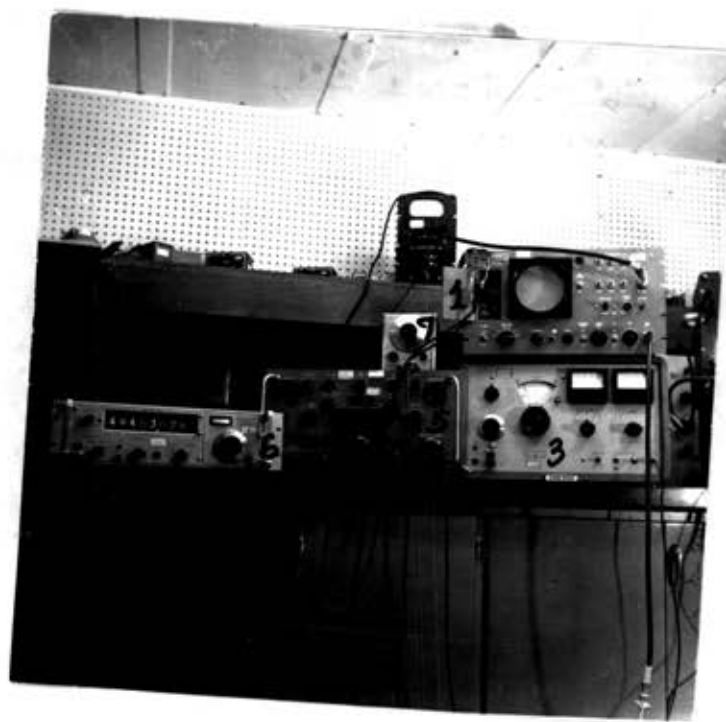
Fig. 18—Shown the connection of the equipments in the SRI Lab.: 1. PANALYZOR SB-12b; 2. PS-12 power supply; 3. 606A Signal Generator; 4. Standard Signal Generator; 5. R-390A/URR receiver; 6. Electronic Counter; 7. 200CD Audio Oscillator (in Fig. is the 204E); 8. Voltmeter and Amplifier.
