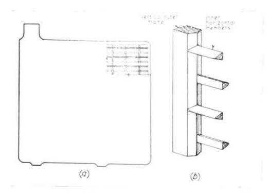
Fig 3 Car Battery Plate.
