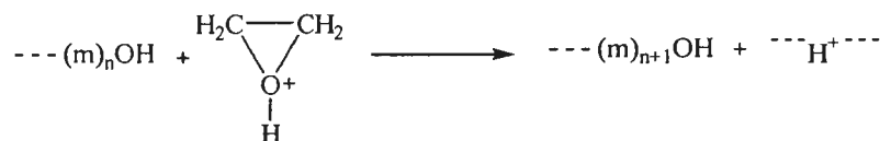
Scheme 2.3 The activated monomer mechanism (AM) in propagation step of CROP.
