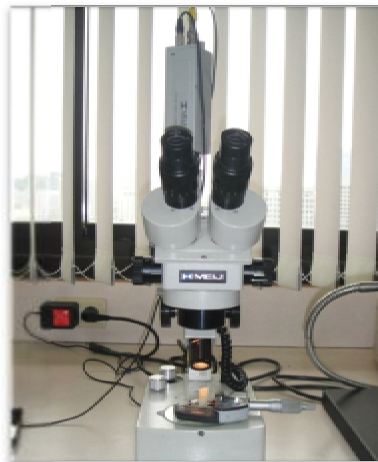
Figure 8. The stereomicroscope with the digital camera
