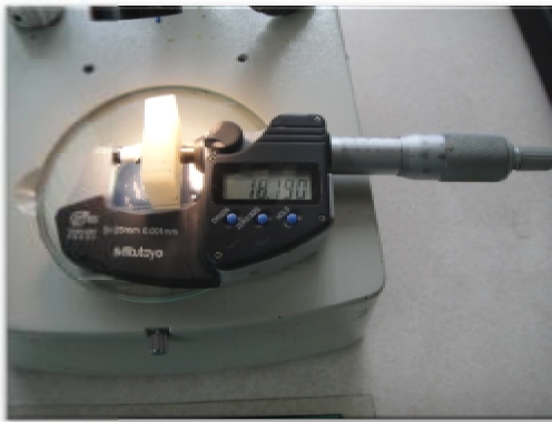
Figure 7. Seating of the specimens using a digital caliper micrometer
