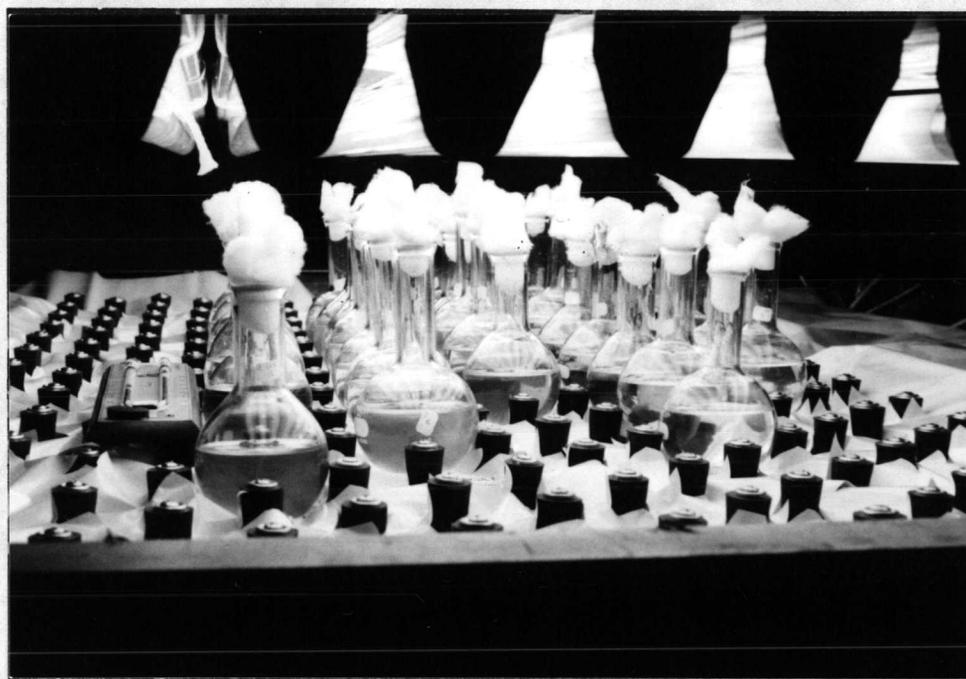
Figure 5. Rotary shaker illuminated with 8 white fluorescent lamps, at 80 rpm shaking speed.
