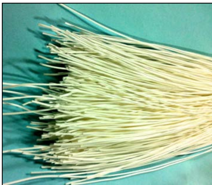
Figure 3.1 PVDF hollow fiber membranes
