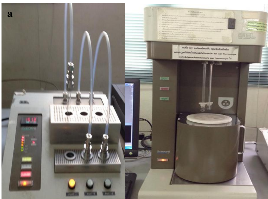
Figure 3. 15 (a) and (b) show heating machine and BET machine for study surface area of nanomaterials
