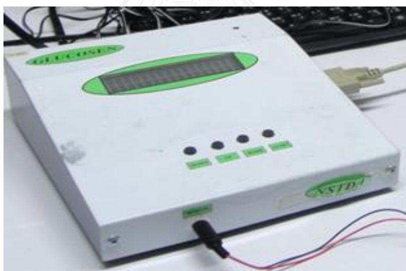
Figure 3. 3 Home made potentiostat machine
