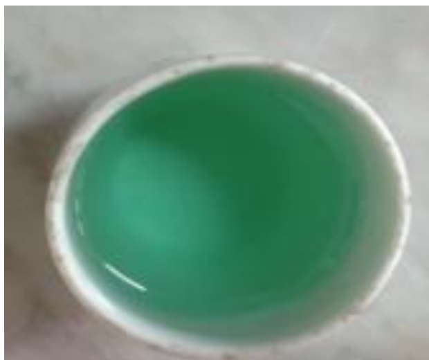
Figure 3. 5 Mixture of Nickel acetate dilute with ethylene glycol and deionized water (1:1)
