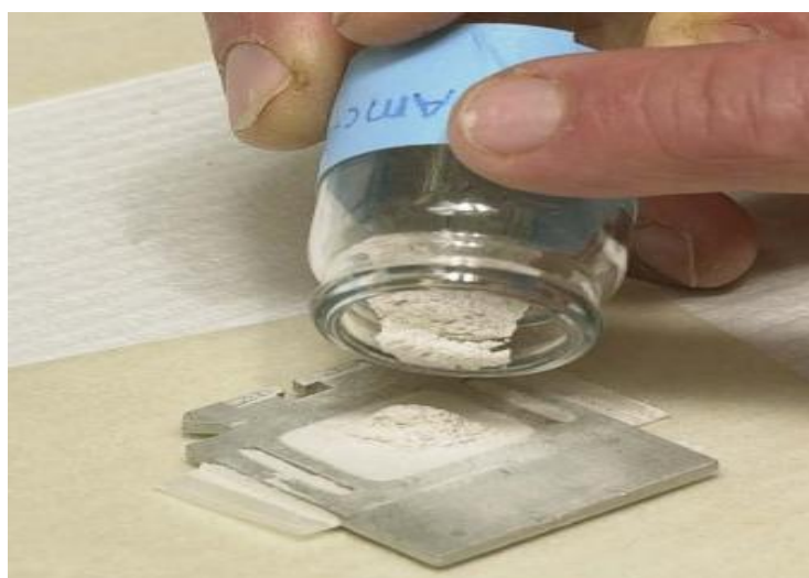
Figure 3. 16 Sample preparation for XRD testing
