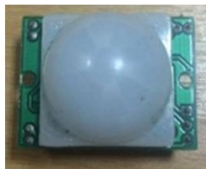
(b) The PIR module with Fresnel lens
