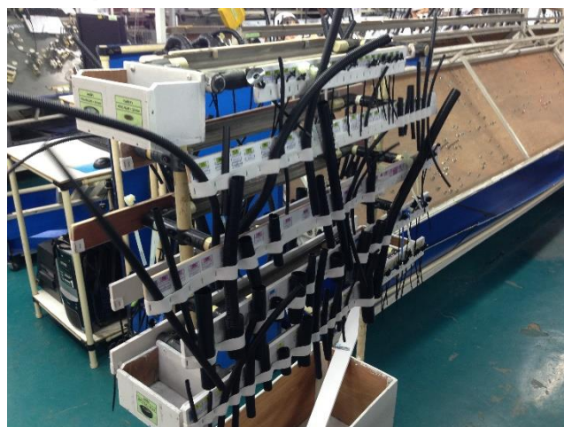
Figure 87: Lay part's Trolley with Five Wasu boards
