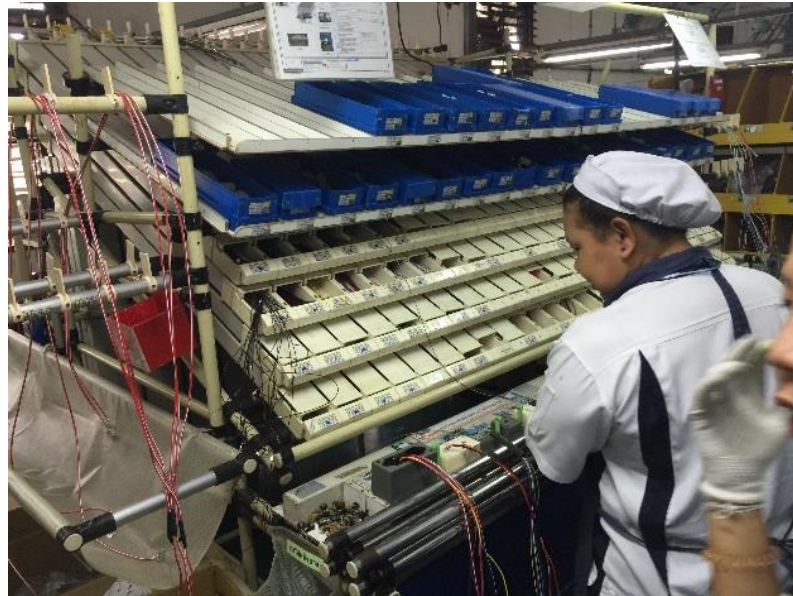
Figure 19: Operator is pre-assembling process of the wires
