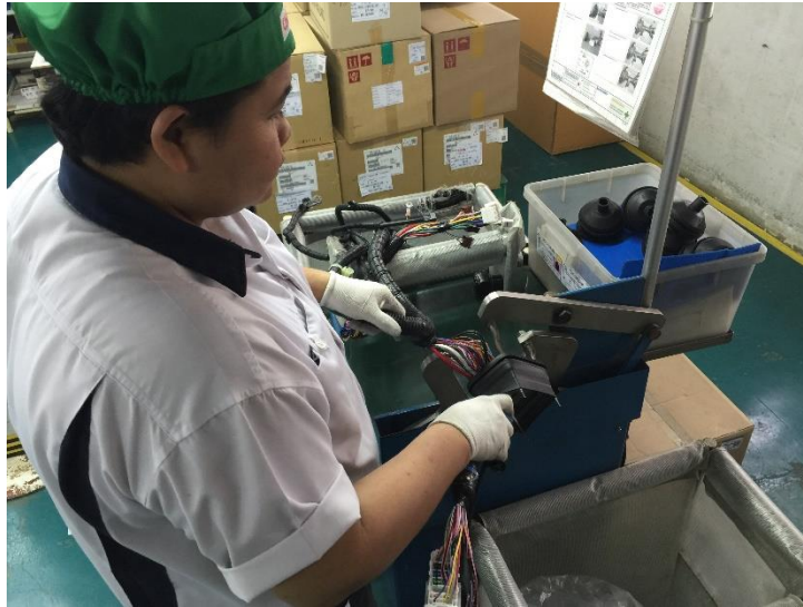
Figure 56: Operator is inserting connectors.
