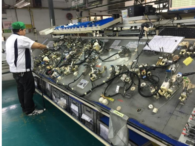
Figure 60: Operator is assembling the harness with checker board
