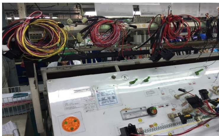
Figure 36: Pre assemble wires are hanging on the bar at assembly board.
