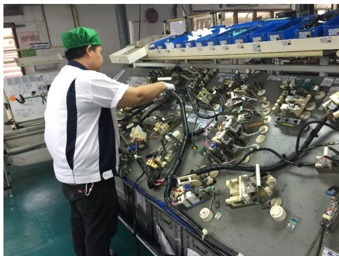
Figure 59: Operator is laying down the harness on the checker board
