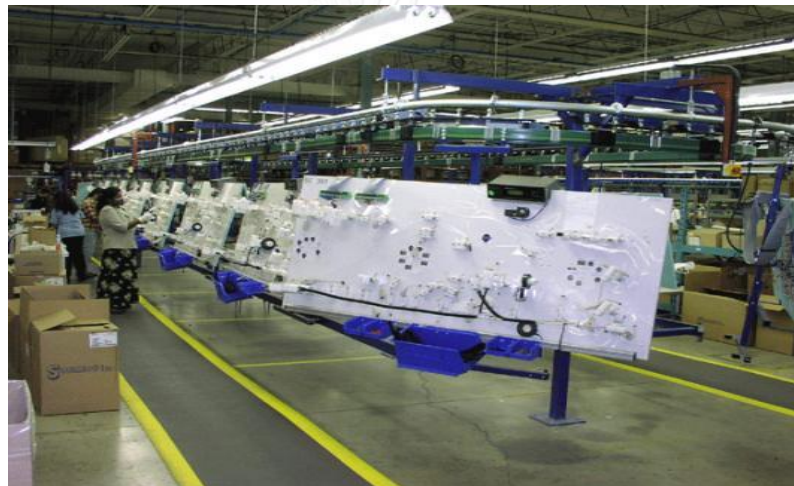
Figure 80: Example of Conveyor line Assembly
