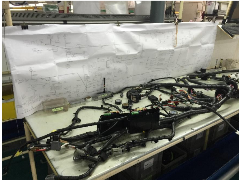
Figure 66: Master Sample of wiring harness
