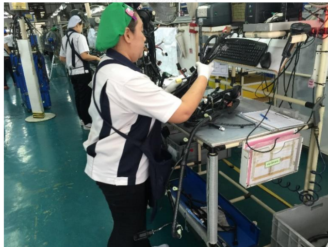
Figure 70: Operator is rolling the harness in to correct form
