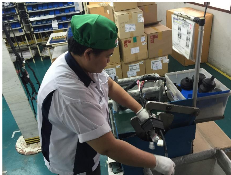
Figure 55: Operator installs the wiring harness to the extending machine
