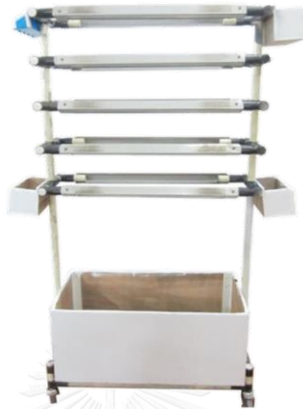
Figure 75: Trolley designed for carrying Wasu boards
