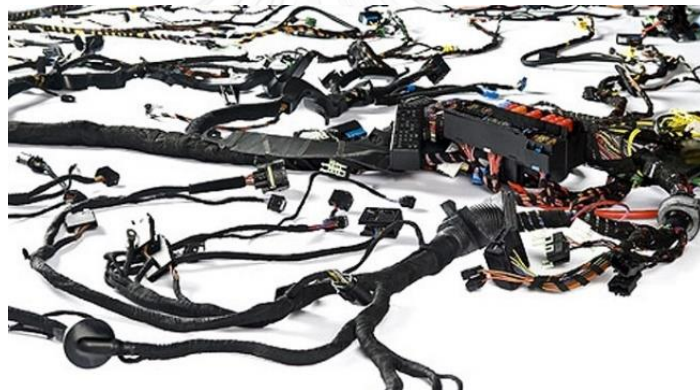
Figure 2: Main wiring harness in vehicles
