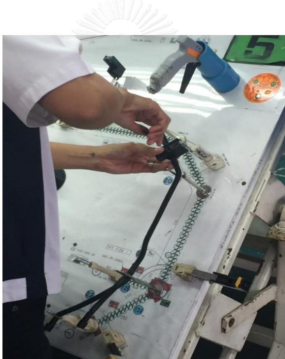
Figure 51: Operator is assembling clips.
