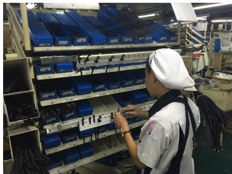
Figure 22: Operator is laying the components on the WASU board
