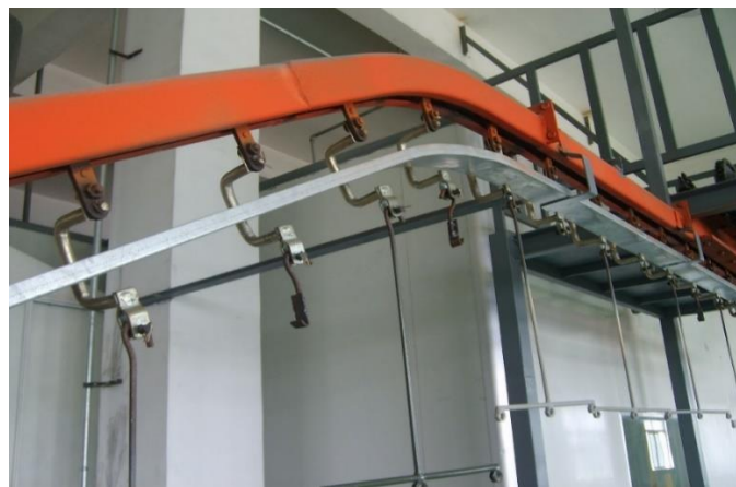
Figure 76: Example of Conveyor line for transporting components to the assembly line
