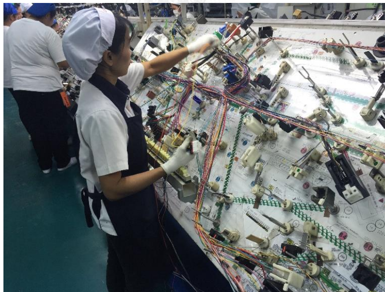
Figure 97: Operator is using Tofix board to lay wire
