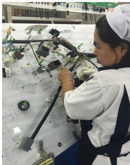
Figure 50: Operator is assembling the tube on the wires.
