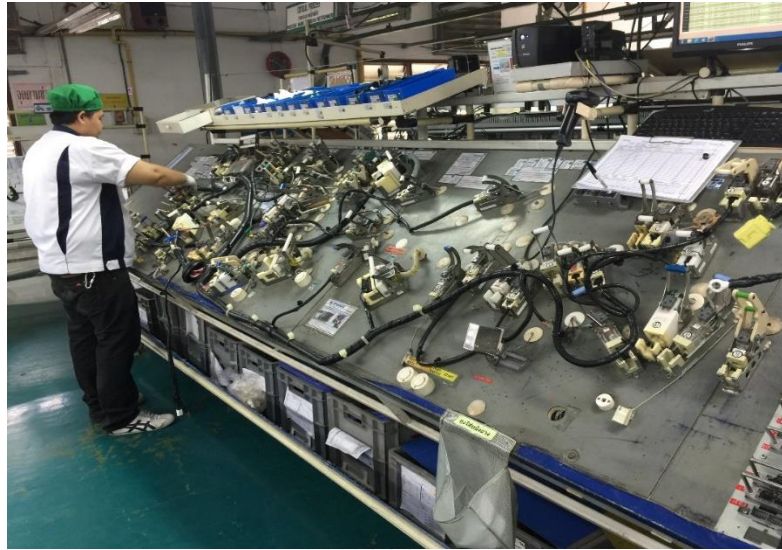
Figure 29: Operator is checking the loom with circuit testing machine
