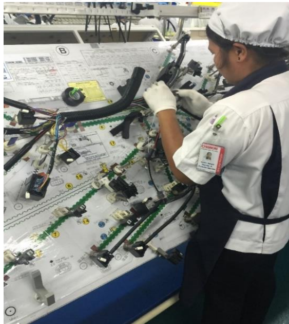
Figure 48: Operator is assembling COTs to the wire.
