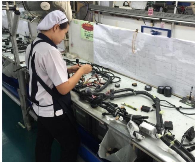
Figure 68 : Operator is inspecting the harness
