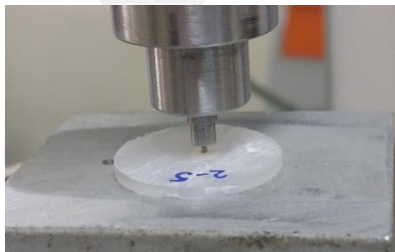
Figure 5 The push out test on a root slice
