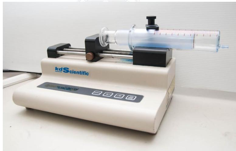
Figure 3.6 A photograph of syringe pump.
