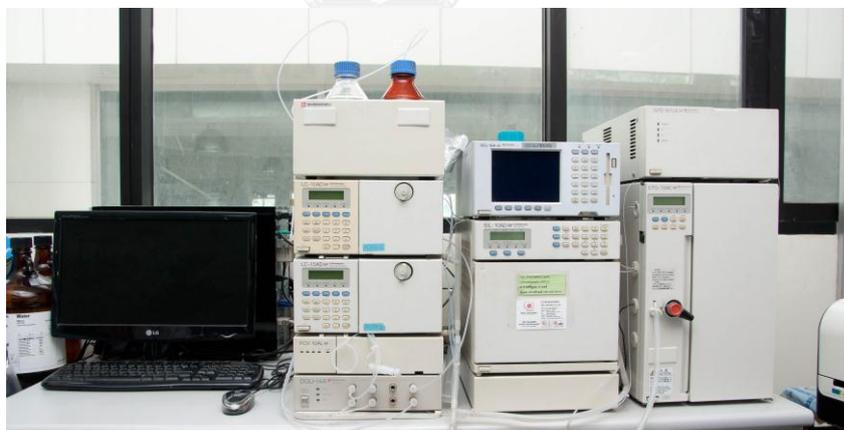
Figure 3.8 A photograph of high performance liquid chromatography
