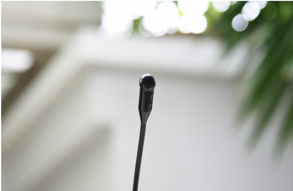
Figure 9 The Cetacean Research™ CR3 Hydrophone: an acoustic tool which was used for receiving all underwater sounds (frequency range: 0.0001-240 kHz, sensitivity: -210 dB, re 1V/ \mu Pa).
