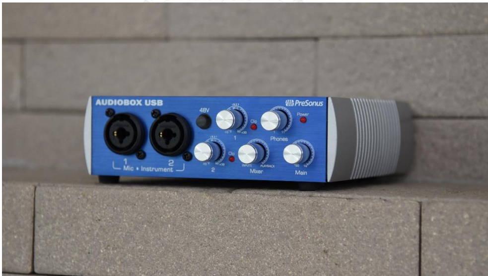
Figure 10 PreSonus AudioBox™ USB: while connecting to the hydrophone and the laptop, this sound recorder was used for recording the underwater sounds (maximum sampling rate = 44.1 kHz).
