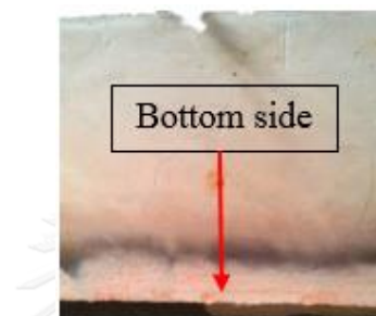
Figure 3.8 The slab after exposure to fire.
