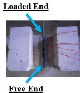
Figure 3.4 CFRP rod and epoxy applied in the groove.
