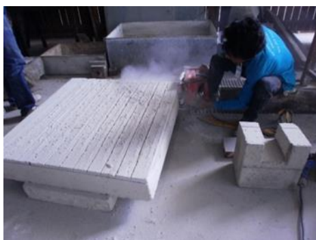
a) Cutting lines on surface of slab b) The surface after removing weakened layer
