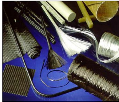
Figure 2.2 Assorted FRP products used for civil engineering structures [15].
