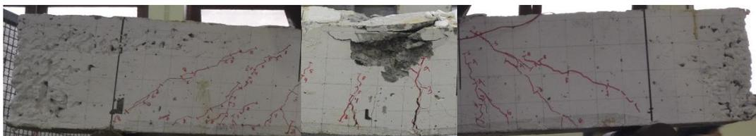
Figure 4.32 Crack pattern of beam NN2 at ultimate load
