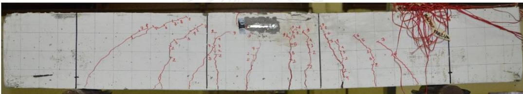
Figure 4.35 Crack pattern of beam RFA-251 at ultimate load
