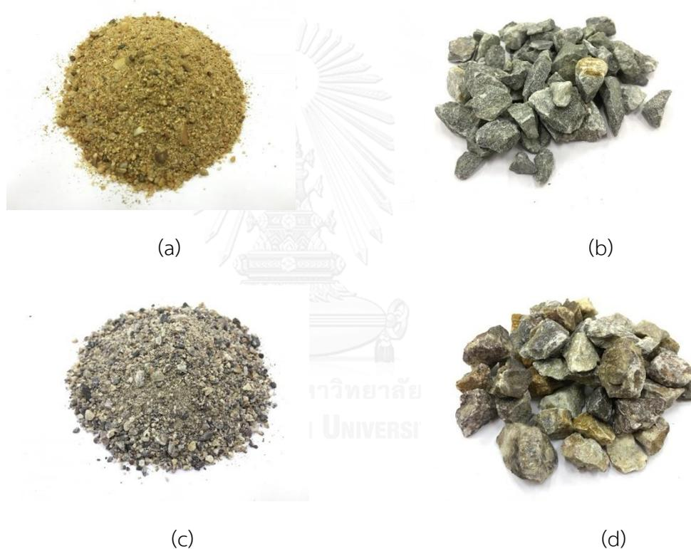
**Figure 3.1** Visualization of aggregates (a) Natural sand (b) Gravel (c) Barite sand, and (d) Barite stone.
