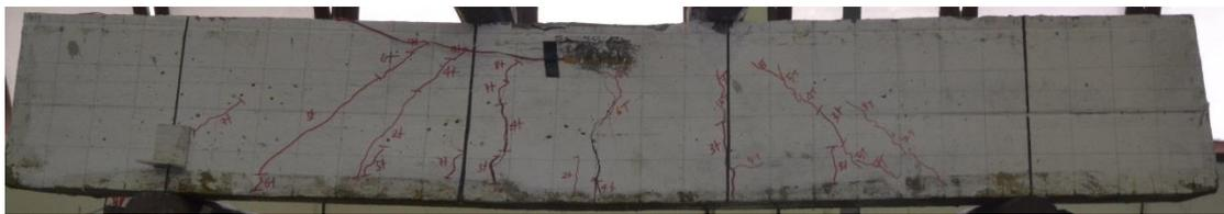
Figure 4.31 Crack pattern of beam NN1 at ultimate load
