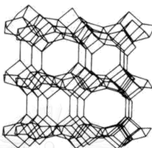
Fig 2. 13 Unit structure of zeolite
