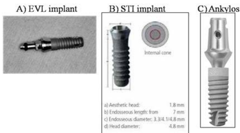
Figure 2.4 Images of implants blasted by \text{Al}_2\text{O}_3 . The EVL implant, one-step, cylindrical, self-tapping endosseous screw-shaped implant made of grade 2 titanium(A), The STI implant produced from grade 4 titanium (B), The Ankylos implant (C)[55-57].
