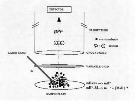
Figure 6 Principle of MALDI-TOF-MS, where mH=matrix, M=analyte, mH\*= excited matrix molecule. The ions are separated in a flight tube where small ions travel faster than large ions, and thereby reach the detector first.
