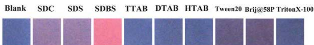
Figure 1.18 Photograph of PDA coated paper derived from primary amine (1% w/v) after being dipped in a solution of SDC, SDS, SDBS, TTAB, DTAB, HTAB, Tween 20, Brij@58P and Triton X-100 (500 mM).
