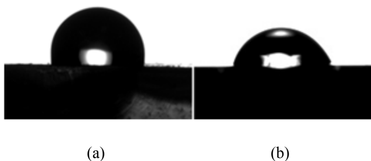
Figure 3.1 Contact angles of (a) untreated PDMS and (b) oxygen plasma-treated PDMS surface.
