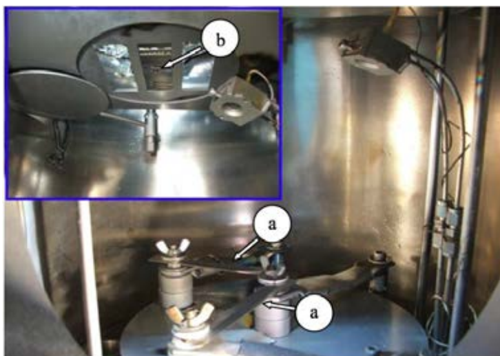
Figure 2.6 Instrument for cathode deposition. (a) tungsten boats and (b) 2 mm wide fingers of a shadow mask.
