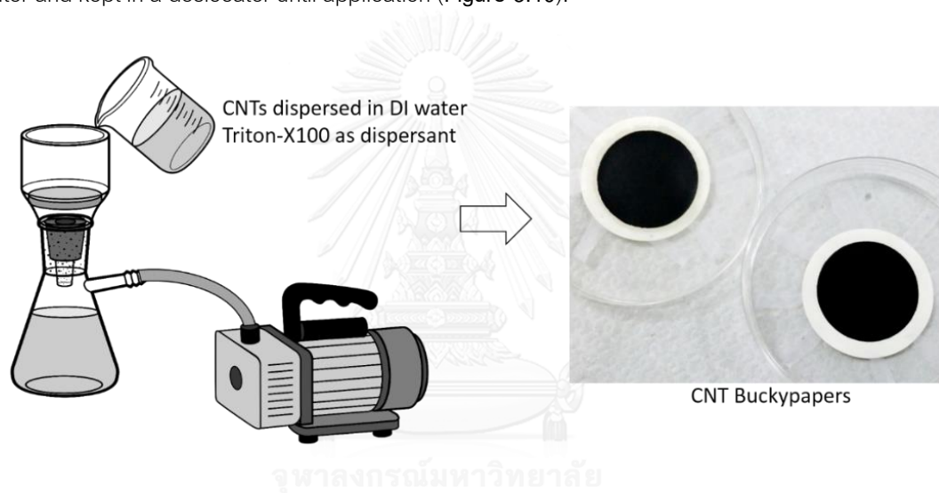
Figure 3.10 CNT Buckypaper preparation via vacuum filtration
