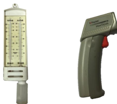
Figure 12 Mason's hygrometer (left) and infrared thermometer (right)
