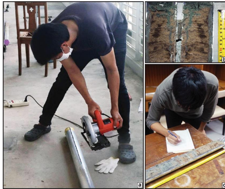
Figure 3.6 Pictures showing core sample; a) sample core was cut lengthwise; b) sample core was divided into two sides longitudinally; and c) core was recorded stratigraphy.
