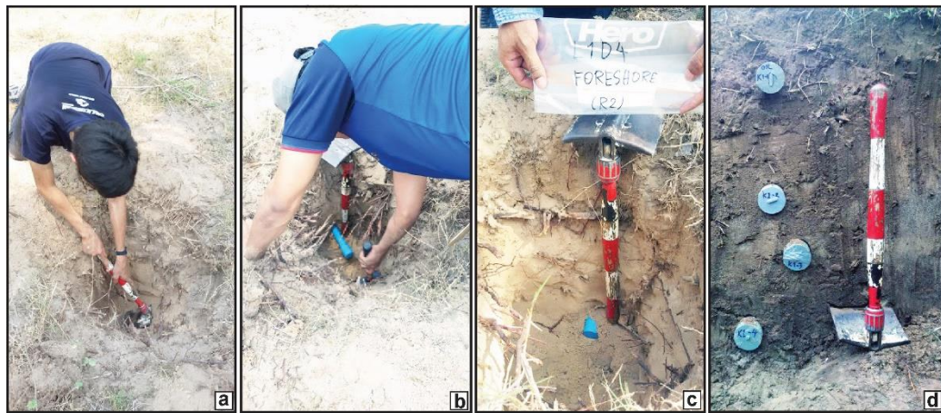
Figure 3.8 Pictures showing collecting OSL samples; a) pitting a small pit; b) and c) OSL sample was collected by PVC tube; and d) collecting OSL samples at natural trench.
