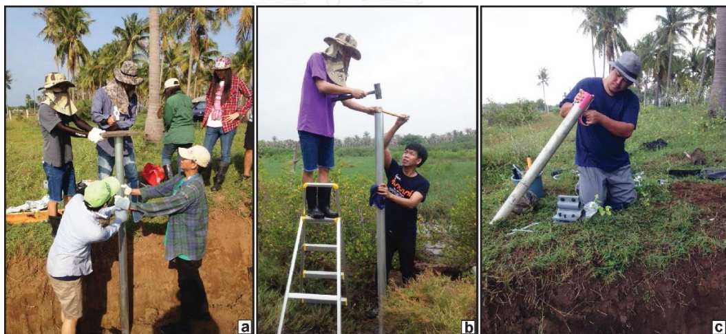
Figure 3.5 Pictures showing collecting sample by percussion coring; a) and b) aluminium tubes were applied to collect ancient storm samples; c) core sample obtained in site was sealed before transporting to laboratory.
