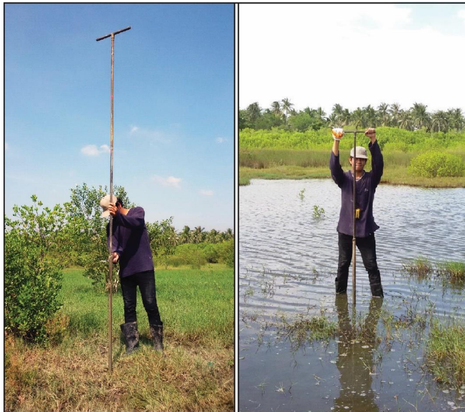
Figure 3.3 Gauge core using for detecting the ancient storm deposits.
