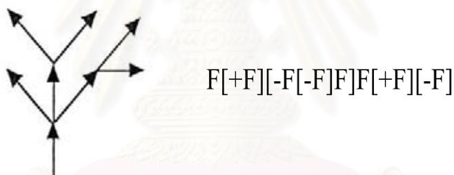
Figure 3.5: Bracketed string representation of an axial tree.
