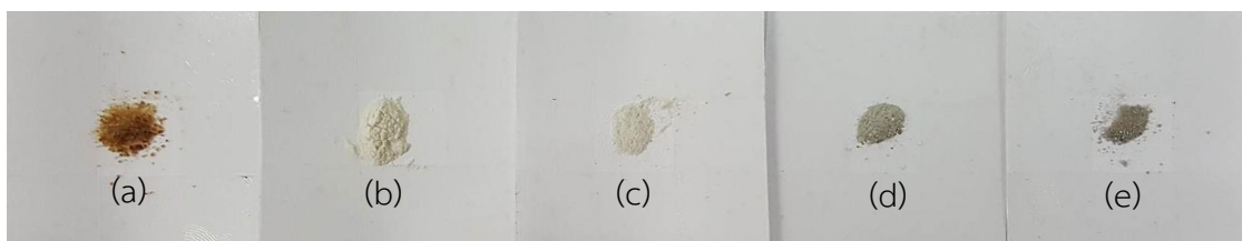
Figure 27 The appearance of spent \text{Al}_2\text{O}_3 and P-modified \text{Al}_2\text{O}_3 catalysts;
