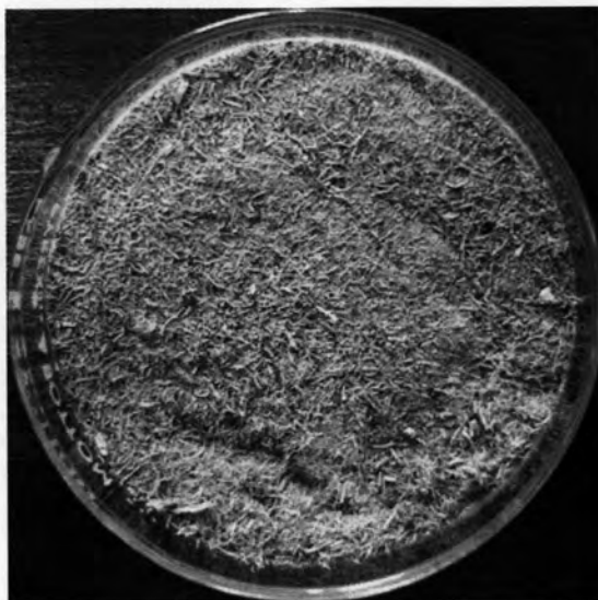
Figure 5 Fiber residue of durian fruit hulls after polysaccharide gel (PG) extraction, a starting material for the isolation of microcrystalline cellulose (MCC).
