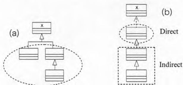
Figure 7.2: The effects of generalization (a) and dependency (b) on changeability [47]
