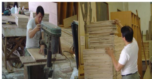
Figure 3-7: Drilling and Edging
