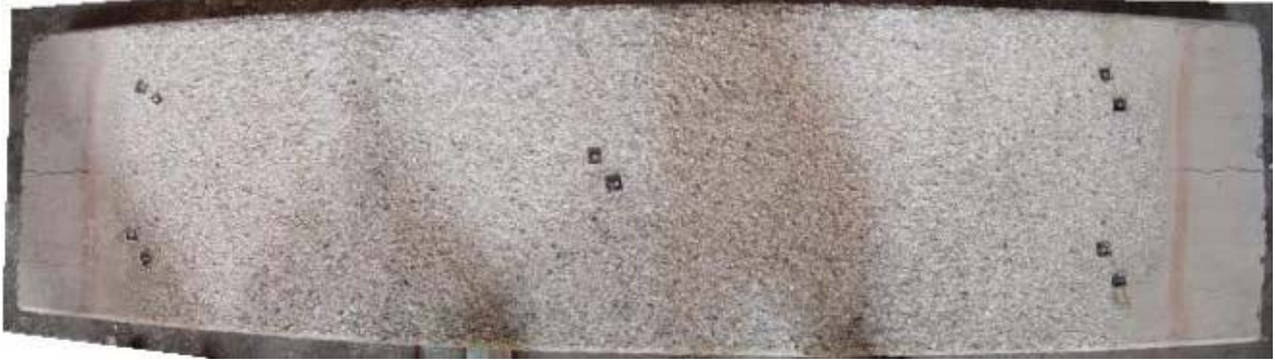
Figure 3.21 LB03 after fire test
