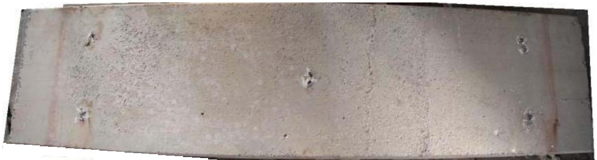
Figure 3.13 TB02 after fire test
