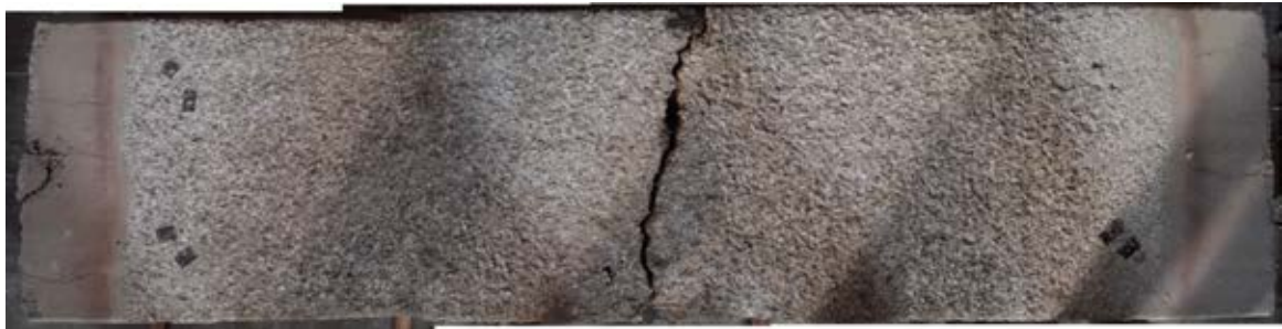
Figure 3.19 LB01 after fire test
