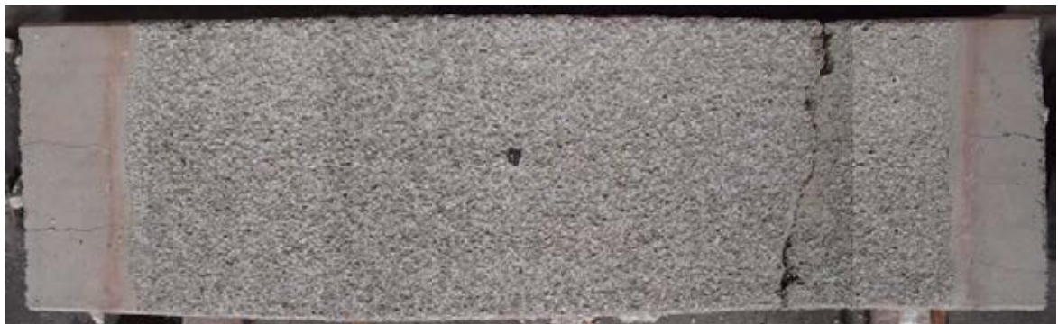
Figure 3.14 TB03 after fire test
