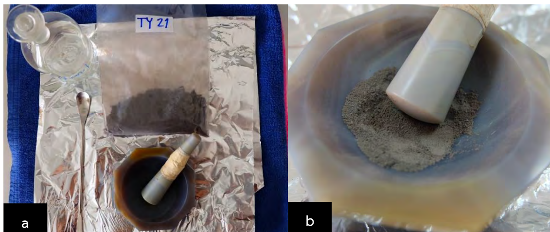
Figure 3.7 (a) Preparation for rock grinding by using agate mortar.
