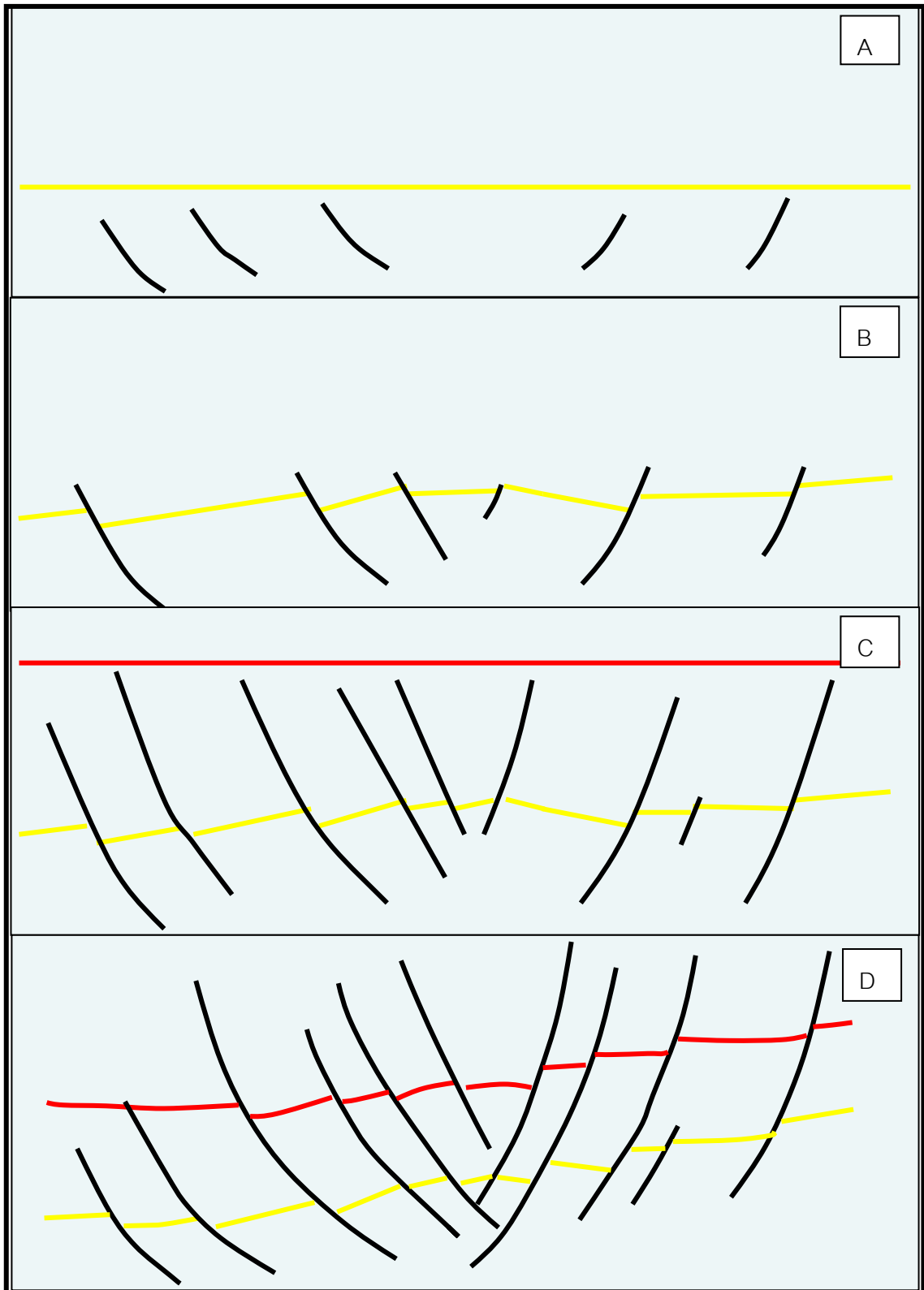
Figure 4.1 Restoration model of horizon X and horizon Z. (A) Flattened horizon Z (B) Occurring of faults in horizon Z (C) Faults continued to activate then horizon X deposited (D) Faults reactivated into horizon X.
