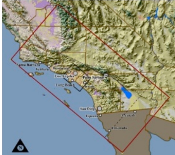
Figure 2.5 Location map for the TeraShake simulations. The red rectangle depicts the simulation area. The black rectangle depicts a section of the Los Angeles basin. The dotted line depicts the part of the San Andreas Fault that ruptured in the TeraShake simulations. (Olsen et al , 2006)
