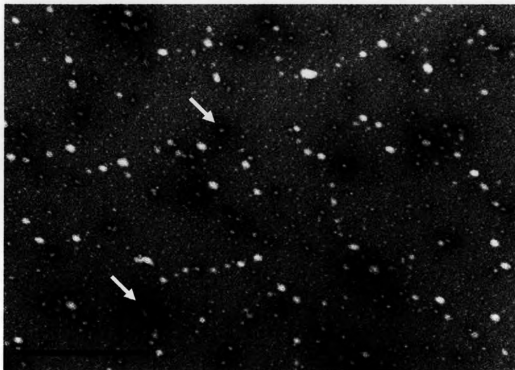
Figure 9 TEM image of 5:1 CSA/DNA S nanoparticles. Bar represents 1 \mu\text{m} . Total magnification is X39600.
