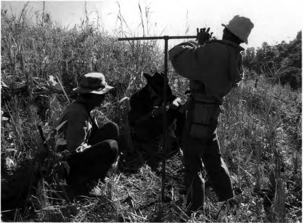
Figure 3.11 Soil samples are collected using hand auger nearby a landslide scar at Nam Phi Village, Thung Chang District, Nan Province for laboratory test.
