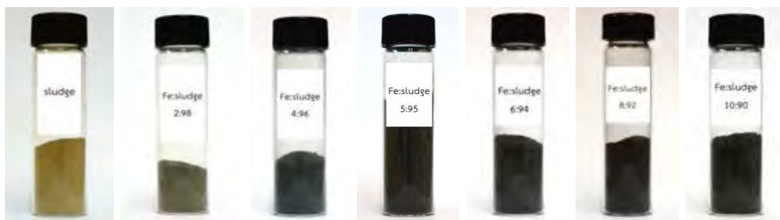
Figure 4.1 Pictures of tap water production sludge and the modified sludge with different iron:sludge ratios.
