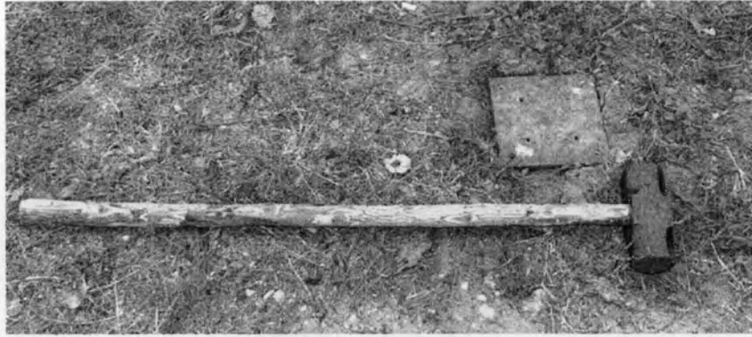
Figure 4-2 A 10 lb sledge hammer and a plate steel used as seismic source
