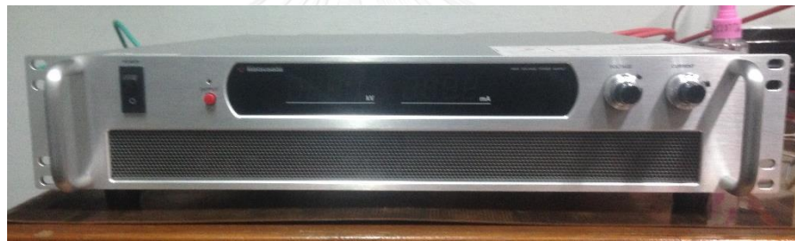
Figure 3.3 Solid state HV Power Supply for the experiments of floating-particle configuration.
