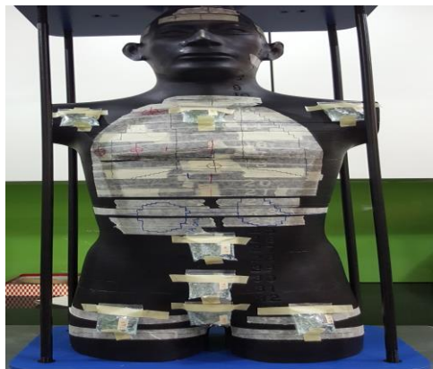
Figure 3.9 The male Alderson RANDO phantom
