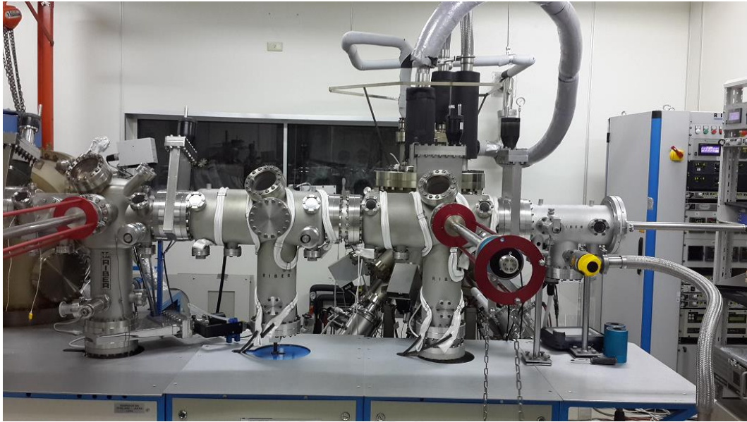
Fig. 3.1 COMPACT-21 MBE system at Semiconductor Development Research Laboratory, Chulalongkorn University
