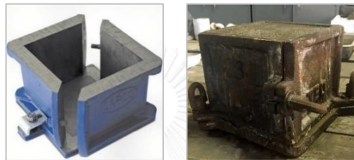
Figure 3.2: Standard concrete mold of specimen.
