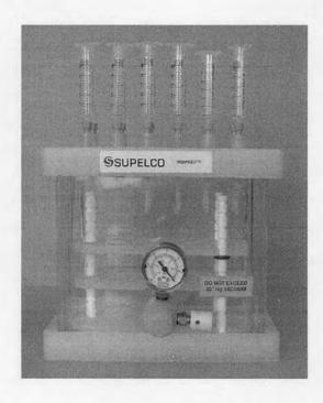
Figure 3.1 Visiprep TM SPE Vacuum Manifold.
