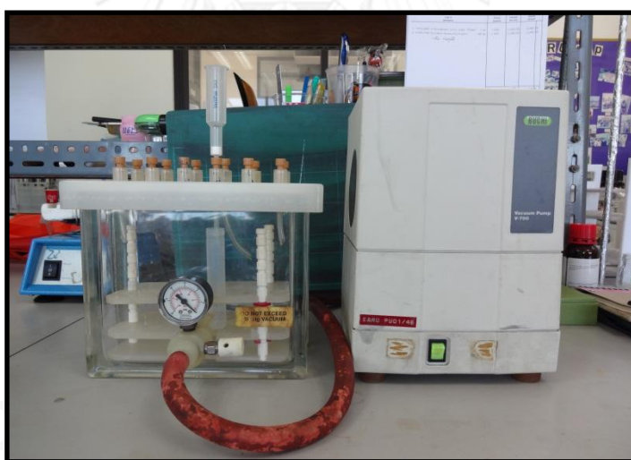
Figure 3.1 Photograph of vacuum manifold system.
