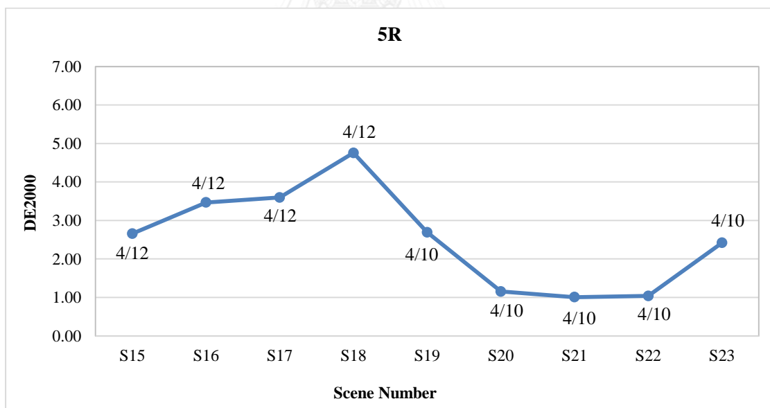
Figure 6.55 Colour differences between calculated and measured CIELAB values across scenes 15 to 23 for the wheel's Munsell Hue 5R.
