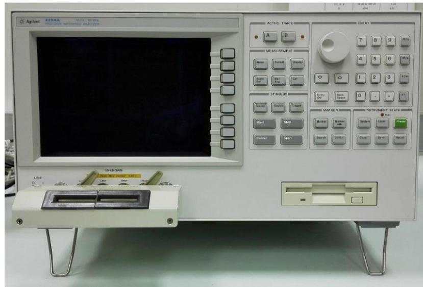
Figure 4.13: Impedance analyzer (Agilent 4294A).
