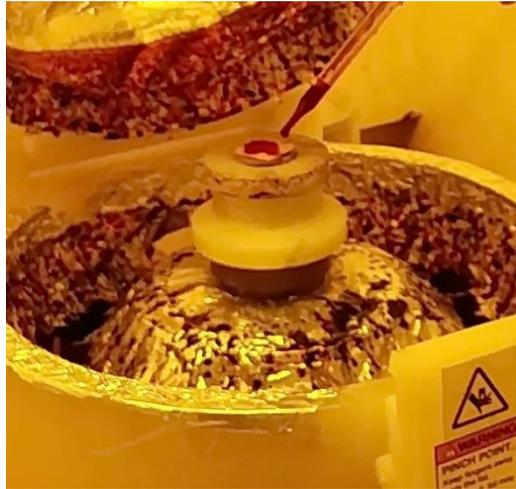
Figure 4.5: Spin coating the substrate with the photoresist.
