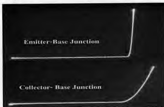
Figure 9. (I,V) characteristics of emitter-base and collector-base junction with the third terminal opened I: 2 mA/div, V: 1 volt/div
