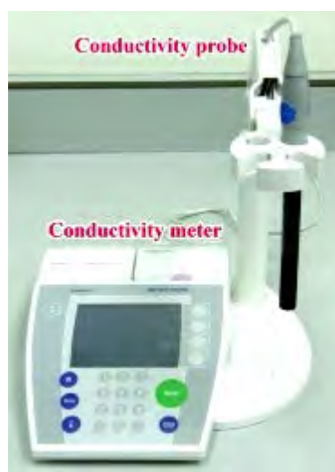
Figure 3.3 The conductivity meter and conductivity probe for electrical conductivity test.
