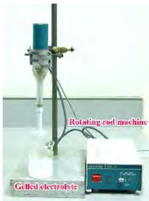
Figure 3.1 The setting of instruments for the gelled electrolyte preparation.
