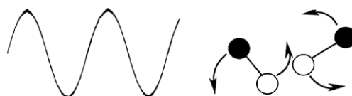
Figure 1.9 Dipolar molecules which try to align with and oscillating electric field.
